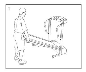
Move your right hand to the position shown and hold the treadmill firmly. Press out on the storage latch. Raise the treadmill until the storage latch closes over the catch. Make sure that the storage latch is fully engaged over the catch.
